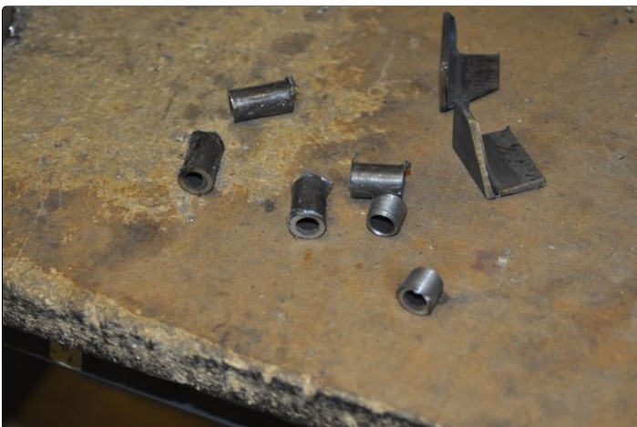
1. I cut short pieces of pipe and welded them to the back of the rack parts as a guide and mounting point for the threaded rod.
