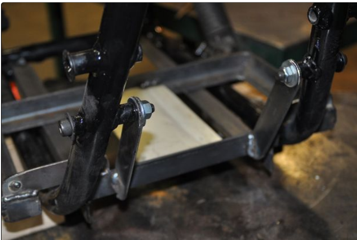
1. Tabs connect lower battery rack to frame of cycle.
