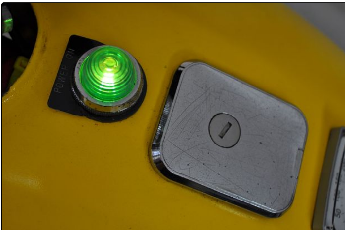
1. Green power indicator light showing that the cycle is ready to go!
