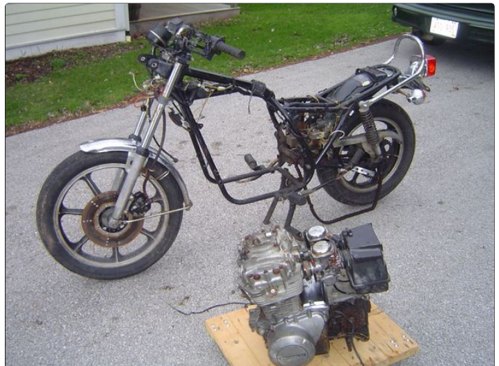
1. Donor bike de-ICE'd. 2. Engine and transmission removed. They didn't work. I got a few bucks on Craigslist for them. 3. Notice that the cycle has twin lower frame members. This is a good start for a "tray" to mount the motor and batteries. 4. The upper part of the frame is a single tube down the center. It somewhat limits battery location. 5. Please note that I saved the gas tank. While an electric motorcycle doesn't NEED a gas tank, it looks much cooler with one! 6. The stock chain was but off and later replaced with one that fit standard machine sprockets.
