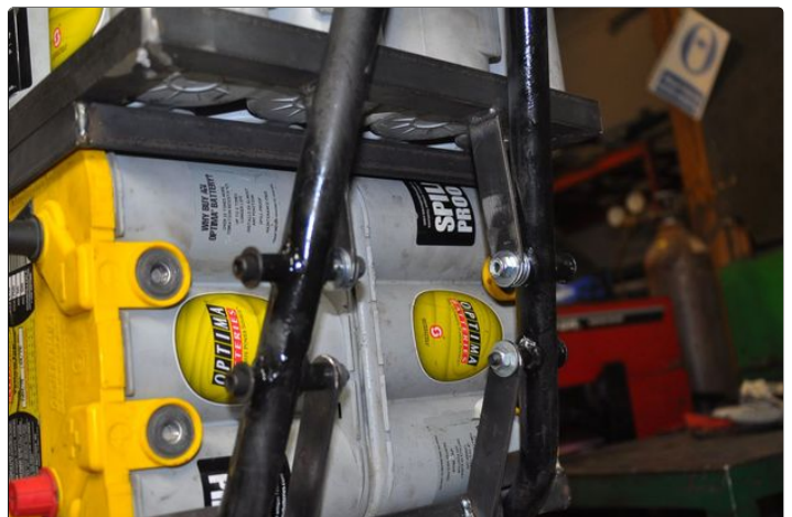
1. Tab connects the middle rack part to the frame of the cycle.
