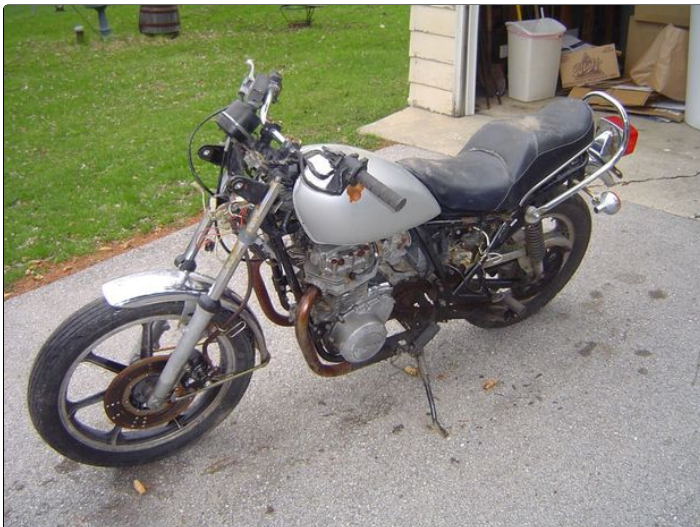
1. My motorcycle as it was originally. Dented gas tank, one muffler missing, broken throttle cable, missing headlight, and rust. In retrospect, I would have picked up a frame in better general condition.
