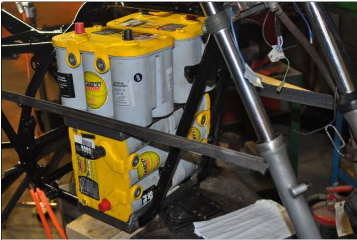
1. Scrap pieces used to temporarily support the upper two batteries to insure that everything is still lining up.
