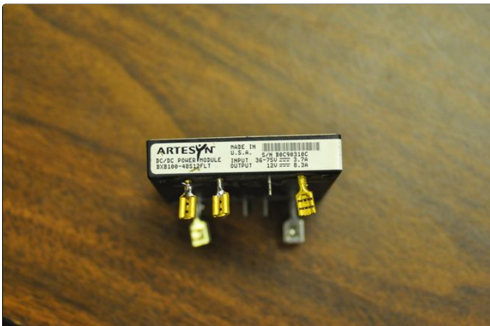
1. This DC/DC converter will take the 48 volts from the main batteries and convert it to 12V to run the headlight, taillights, horn, and other 12V items on the motorcycle. 2. This DC/DC converter is 2" square by 1/2" thick, and replaces weight and bulk of a separate 12V battery and charger.
